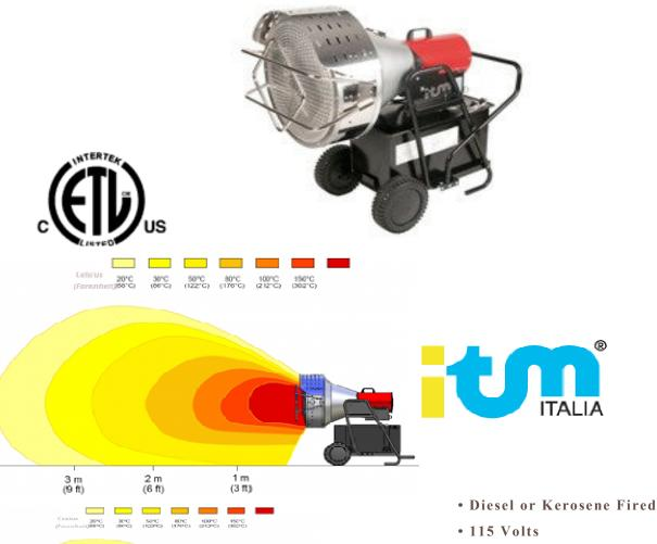
The V40 uses advanced infrared technology, the flame inside the insulated cone heats the front disk which serves two purposes, to radiate the heat and also as a catalytic converter reducing emissions to near zero.
