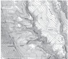
e. Valley – A valley is level ground bordered on the sides by higher ground. Contour lines indicating a valley are somewhat U-shaped.
