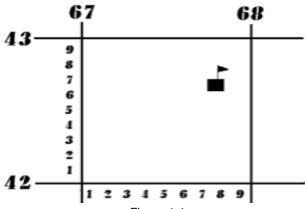
For example: Grid reference 678427 is given, the easting is 678 or 67 and 8/10, and the northing is 427 or 42 and 7/10.
