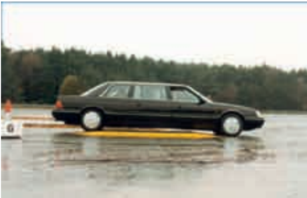
Fig. 4.1 Track trials to examine grounding of vehicles
