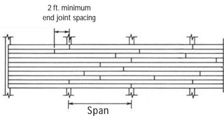
*Simple Spans*--This configuration requires specified length decking and provides shorter spans for the same thickness decking than the random length layout.
