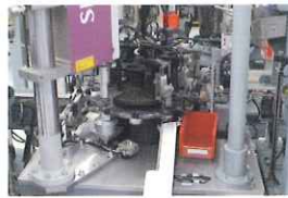
Ultrasonic welding of the nut
