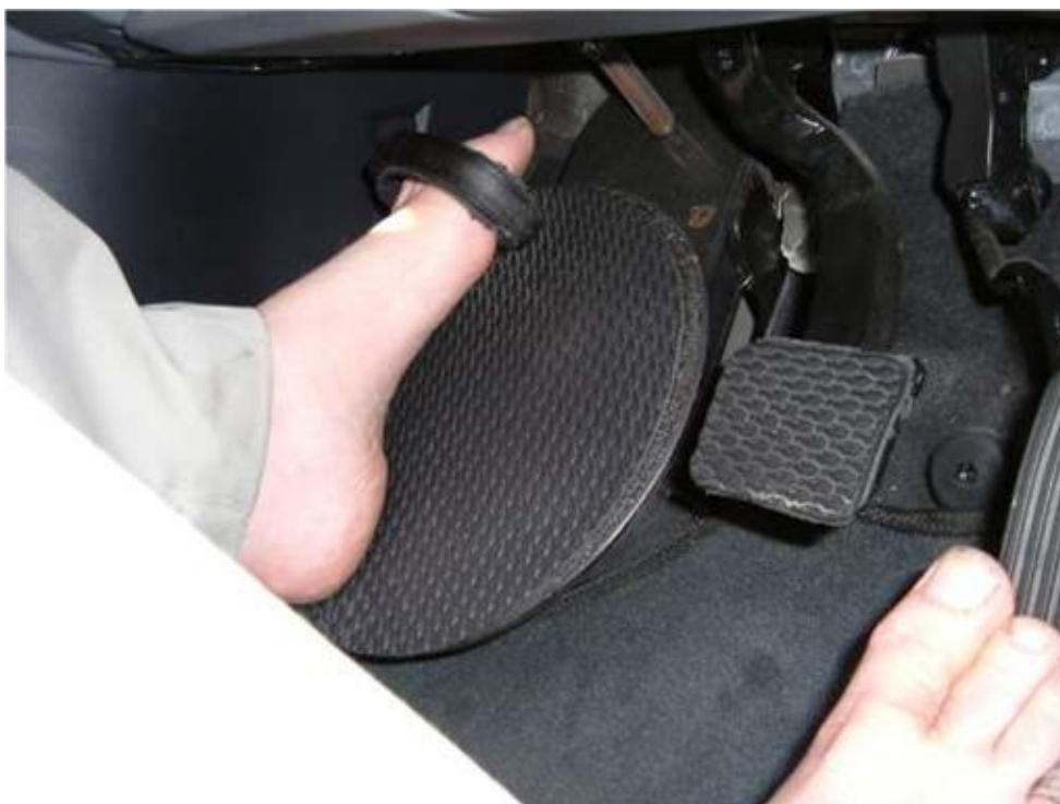
Figure 1 - A steering plate for a thalidomider with short or no arms, costs around £6,000 with an additional £15,000 for other specialist controls and alterations.
