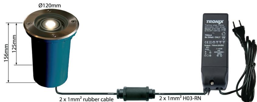
The ground spot 2.5 Watt is standard available in white, warm white and green and with 40° lens. Other lenses available (15°/25°/60°). Ground Spot comes with 2 meter rubber cable 2 x 1mm, which can be connected to the 2 Way Connection Tube (142-007)
