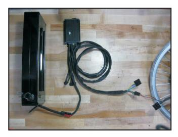
Plug the controller hall cable to the motor hall cable, and then power up the controller with a battery pack. If the controller has an ON/OFF switch, make sure it is ON.
