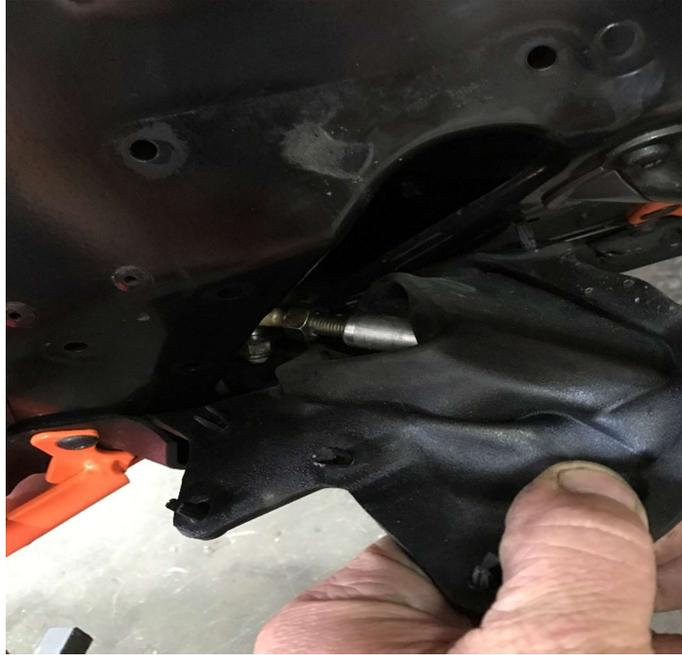
4. Thread the formed tie rods onto inner tie rod end. As a starting point just thread it against the jam nut and then position the bend in the tie rod towards the front of sled as shown in photo.
