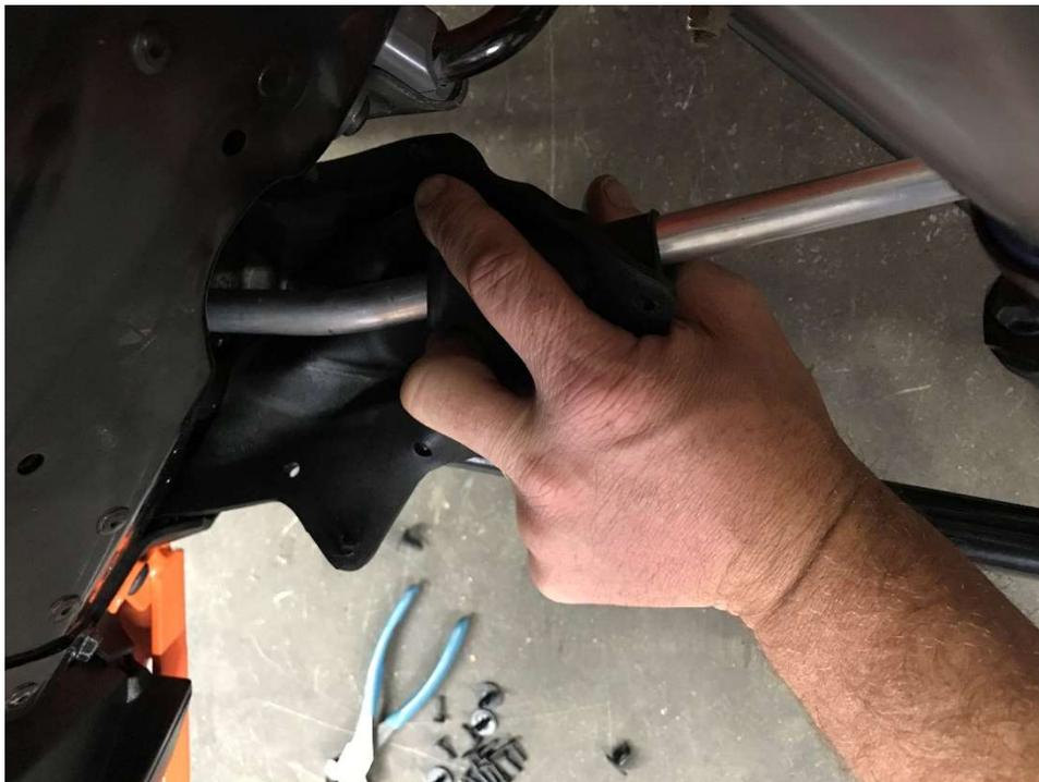
5. Install the outer tie rod ends provided with the kit. Install them so that the amount of threads exposed matches the inner tie rod end.
