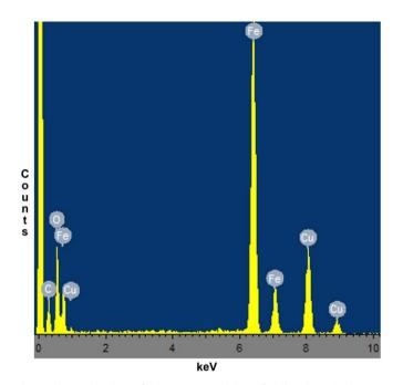
**Fig. 3.** Elemental analysis of the  $Fe_3O_4$  NPs which verified that the main elements in the NPs are Fe and O. Copper (Cu) element was detected as the sample holder is made of Cu and carbon was detected due to the hexane traces on the surface of the  $Fe_3O_4$  NPs.
