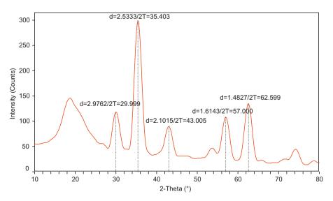
Fig. 2. XRD pattern of synthesized magnetite shows a typical pattern for Fe<sub>3</sub>O<sub>4</sub> NPs crystal structure with six characteristics peaks.
