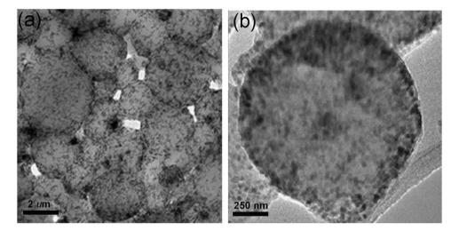
**Fig. 6.** TEM micrographs of NMNP prepared with 100 mg PLLA, 15 mg, Fe<sub>3</sub>O<sub>4</sub> NPs and 7.5 mg noscapine, (a) bar =  $1.0 \mu$ m, shows that bulk of the nanoparticles synthesized are of uniform size with few aggregates, (b) bar = 50 nm scale, a magnified image of shows a spherical shaped NMNP with an approximate size of 250 nm.
