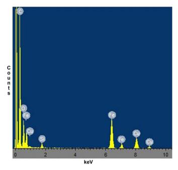
**Fig. 8.** Elemental analysis of the NMNP verified the presence of elements Fe and O on the surface of the polymeric nanoparticles which proved the encapsulation of the Fe<sub>3</sub>O<sub>4</sub> NPs on the surface of the polymer.
