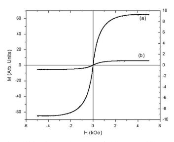
Fig. 5. Field dependent magnetization at 25  $^{\circ}$ C for (a) Fe<sub>3</sub>O<sub>4</sub> NPs and (b) NMNP (prepared with 100 mg PLLA, 15 mg Fe<sub>3</sub>O<sub>4</sub> and 7.5 mg noscapine).
