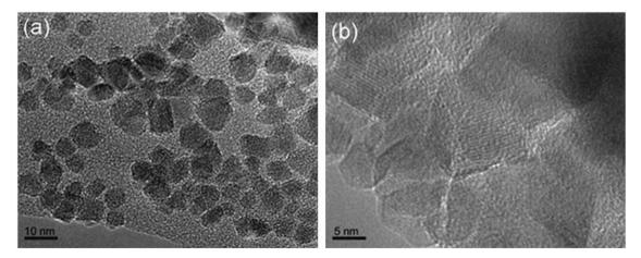
**Fig. 4.** TEM micrographs on synthesized magnetite, (a) bar = 10 nm, shows that bulk of the nanoparticles synthesized are of uniform size with few aggregates, (b) bar = 5 nm scale, a magnified image of shows that an aggregate is a collection of nanoparticles with different lattice structures.
