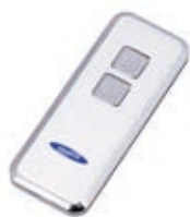
Radiocomando Mini-Novotron 522 Design 2 canali, 433 MHz, KeeLoq-Rolling code.
