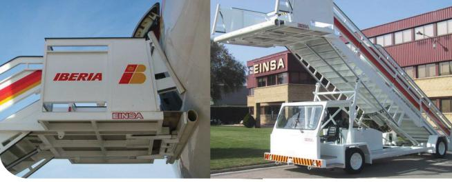
Easy to operate, easy to maintain, the Self-propelled Universal Passenger Step, model EDU-WIDE, has been designed for embarking and disembarking passengers on all aircraft with sill heights ranging from 2.40m to 5.80m (front door of B737 to rear door of A-340) and can be provided with open or closed cabin and optional canopy. The unit incorporates hydrostatic transmission, diesel engine and hydraulic steering in a slide open engine compartment.
