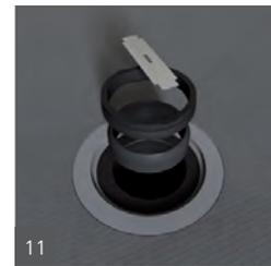
Tighten (squeeze) the rubber caulking gasket firmly with the caulking nut (use a flat headed screwdriver) and finally insert the plastic frame and strainer on top (without adhesive). The frame and drain cover will be held in a grout joint only once tiling commences.
