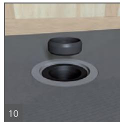
Set up the rubber caulking gasket (with the bevelled side up) around the 2" pipe in the subfloor. The rubber gasket must be flush with the upper end of the 2" ABS or PVC pipe.
