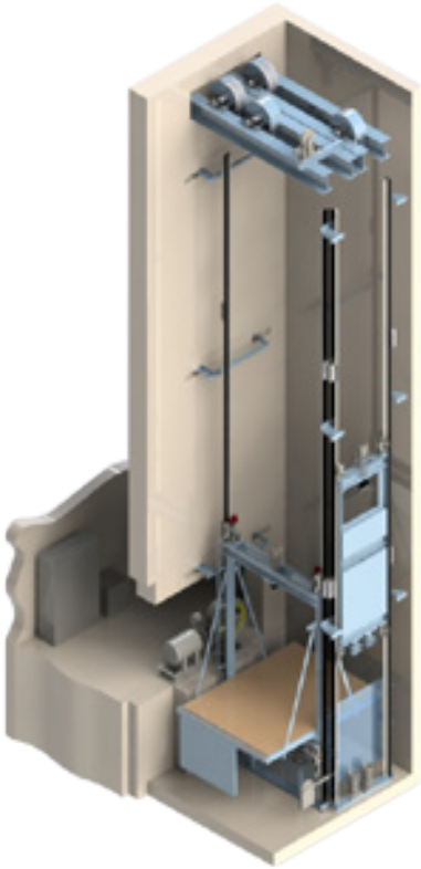
GEARED BASEMENT APPLICATION
