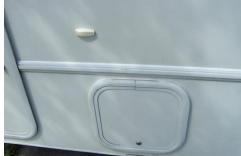
Most of the bins have bullet latches (see above right) to assist in holding the compartment hatches open when loading / unloading the bins.
