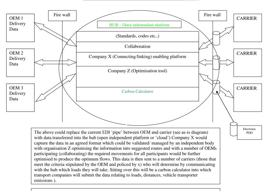
The hub /platform/cloud could be further enhanced through the use of RFID and tracking from factory through to final dealer delivery (and beyond) and include damage survey/claims.
