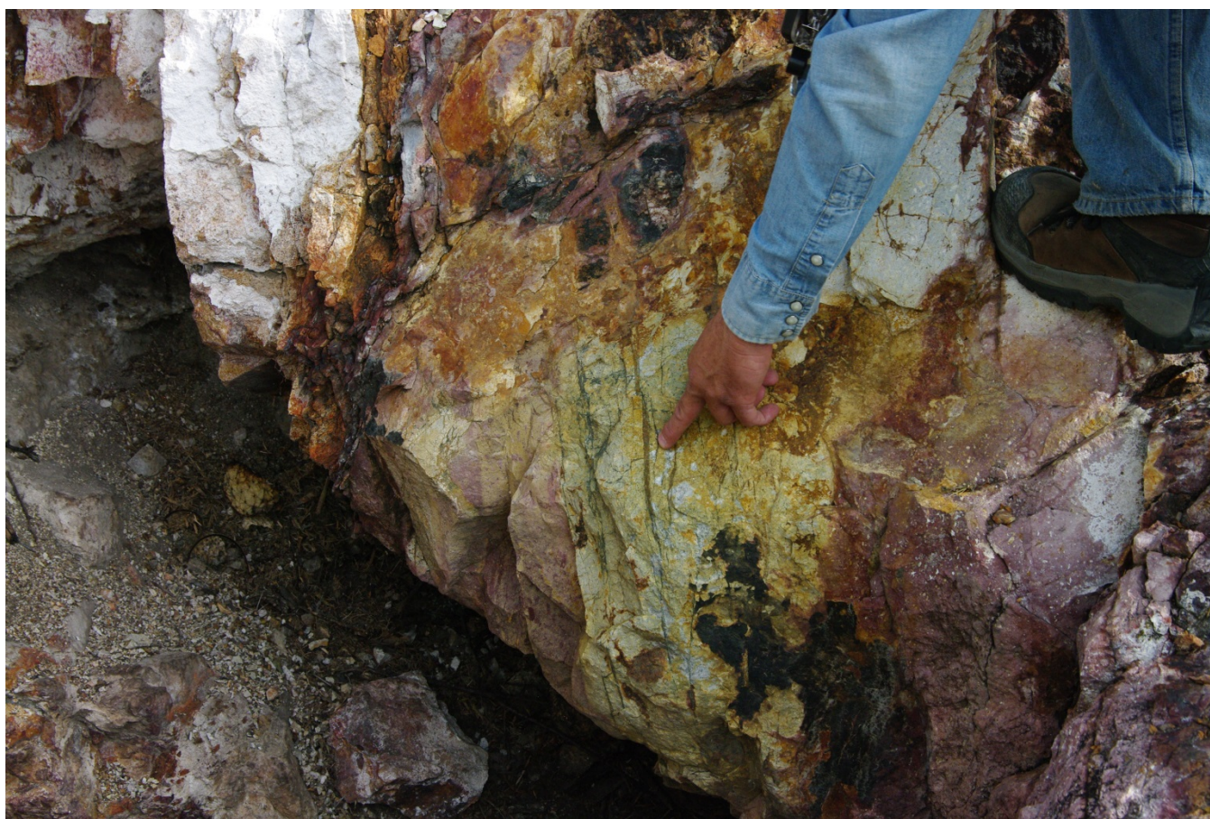
Figure 2: Limited exposures near historic workings-sheeted sulphide veins in monzonite porphyry dyke
