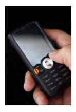
The process of TDMA results in a continuous low frequency pulsing at 8 to 34 Hz. Some phones also have the energy-saving discontinuous transmission mode (DTX), which emits yet a third, even lower frequency that pulses at 2 Hz when the user is listening and not speaking.
