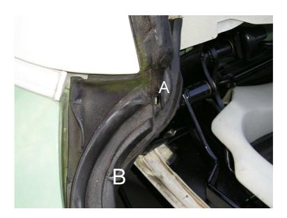
After investigating and curing a water leak into the car – it's important to dry out the wet areas otherwise it's all too easy to end up with serious corrosion in the floor panels. It may be wise to remove the carpet, allow it to dry and refit when you're confident there's no longer a leak. Carefully check the car and lower boot floor – treat any rust with Kurust and finish with a coat of paint.
