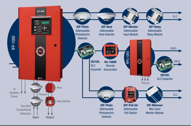
Flexput<sup>®</sup> Circuits - Flexible input or output circuit that you can conveniently program to be used for Notification Appliance Circuits, Auxiliary Power, or as a conventional input circuit. With auxiliary power, it can be selected as constant power, door power, or resettable smoke power. The Flexput circuits provide the utmost versatility without the added expense of additional modules, a perfect fit for retrofitting an existing conventional system when budgets are a concern.
