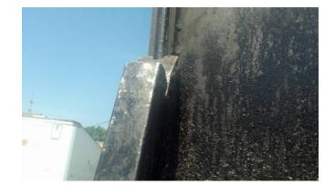
The patented claw has a 3/4" opening that fits most liquid tight seals cleaning off the seal without ever climbing on the truck, and never getting your gloves dirty.
