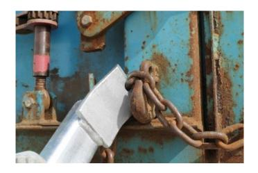
The claw also works great for releasing chains. Sometimes chains can pinch, and be very difficult to remove. The Boom Dog Bar makes the job faster and easier.
