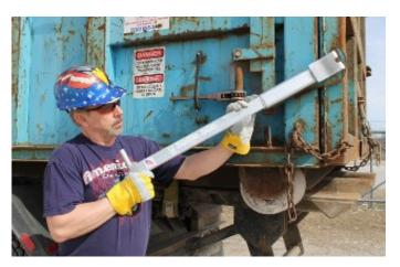
If the door still does not open the bar is designed with an opening to fit the door. The patented punch will kick open the door without ever having to expose your body.
