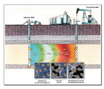
Cross-section illustrating how carbon dioxide and water can be used to flush residual oil from a subsurface rock formation between wells.
