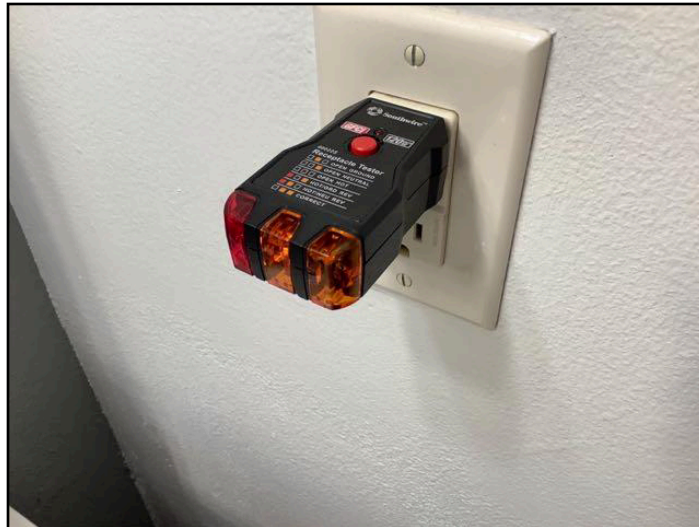
26. Ungrounded GFCI in Bathroom
