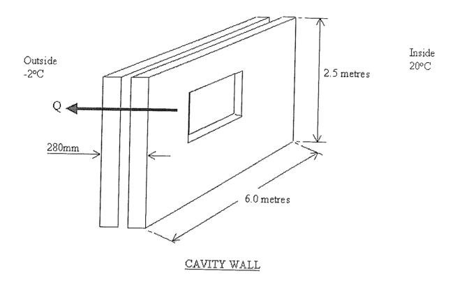
The 'U' value for the blockwork in the wall is  $0.317~\mathrm{W/m^2\,^oC}$
