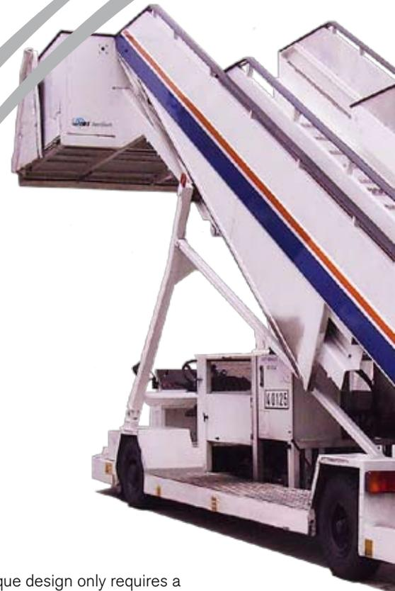
Our unique design only requires a single hydraulic cylinder for step extension and height adjustment simplifying the operation and minimizing the maintenance cost.
