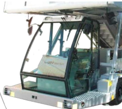
The front mounted, centrally located driver's station provides the operator with an unrestricted view of the aircraft's passenger door when positioning the passenger stairs. Various types of open or closed cabs available.
