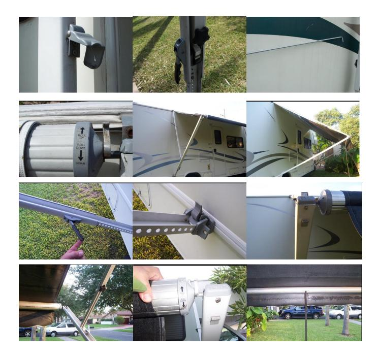
To close the awning: loosen the black knob, depress the grey tab at the upper end of each arm to release the inner arm. Slide the inner arm down towards the RV. Turn the directional lever on the end of the awning tube to the up arrow position. Using the canvas strap and rod, allow the awning to roll itself up. Make sure the main arm is properly seated against the roof of the RV. Tighten the black knobs and close the gray travel latches on the sides of each post.
