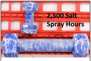
Photos Samples at 2,500 Salt Spray Hours conducted by Assured Testing Services
