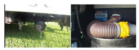
There is also a valve for the shower drain which is closed for travel. It is located on the passenger side of the vehicle just behind the tailpipe, under the RV.
