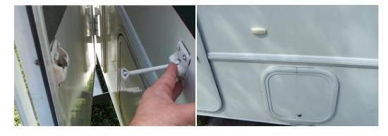
Most of the bins have bullet latches (see above right) to assist in holding the compartment hatches open when loading / unloading the bins.
