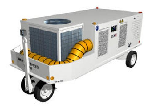
The ACE-HGEU90 Air conditioning and Ventilation Unit provides comfortable aircraft cabin temperatures in all ambient conditions for passenger, cleaning, or maintenance personnel comfort in all types of 12-40 passenger capacity commuter and corporate aircraft. Since the ACE-HGEU90 operates using flood duct air conditioning, aircraft without external connectors may be serviced.
