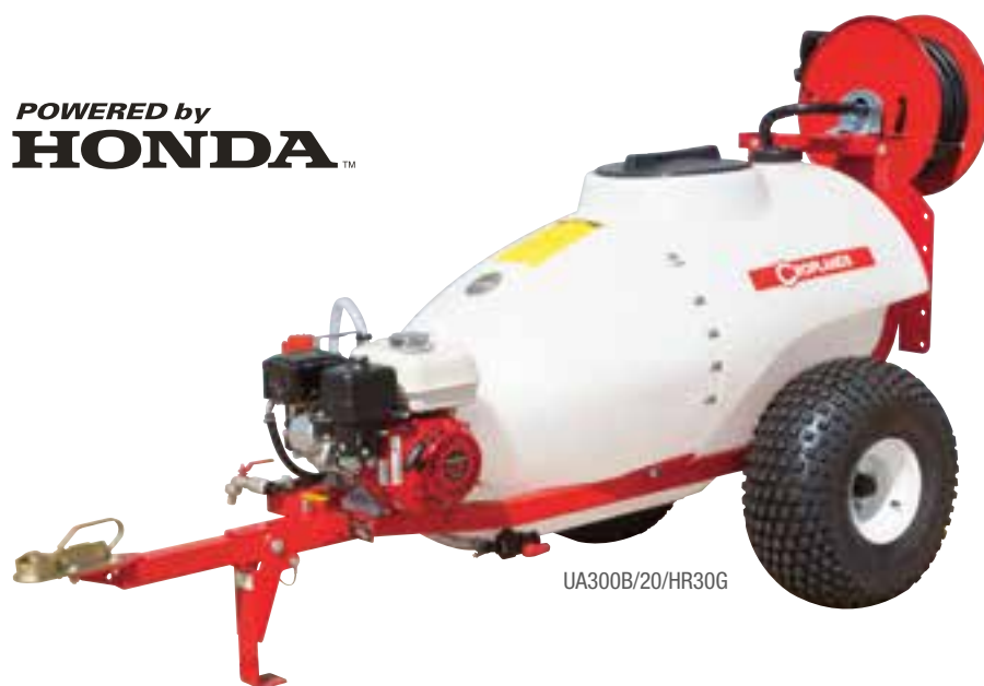
UA300B Trailed sprayer with 30 metres of hose, 25 litre per minute Honda-powered pump and spray gun – ideal for nurseries and greenhouses where hand-gun spraying is needed.
