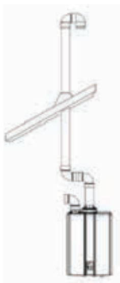
Vertical termination room air configuration
