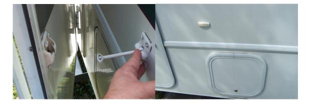
Most of the bins have bullet latches (see above right) to assist in holding the compartment hatches open when loading / unloading the bins.
