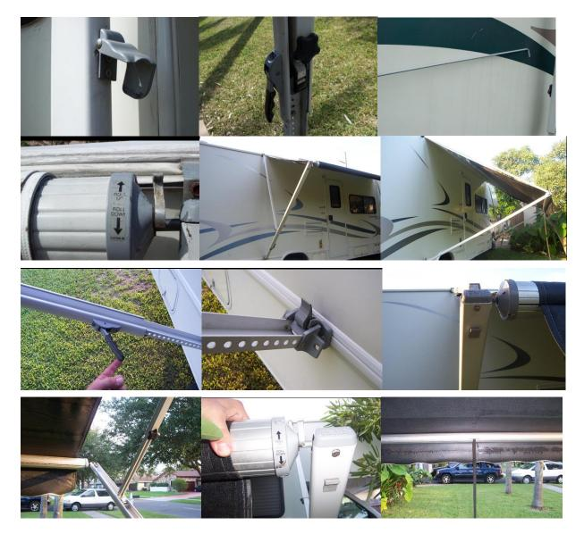
To close the awning: loosen the black knob, depress the grey tab at the upper end of each arm to release the inner arm. Slide the inner arm down towards the RV. Turn the directional lever on the end of the awning tube to the up arrow position. Using the canvas strap and rod, allow the awning to roll itself up. Make sure the main arm is properly seated against the roof of the RV. Tighten the black knobs and close the gray travel latches on the sides of each post.
