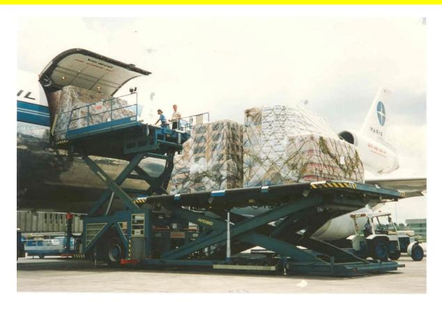
UNIVERSAL LOWER & MAIN – DECK, CONTAINER / PALLET LOADER Wide front and main platform for transversal handling of 125" ULD
