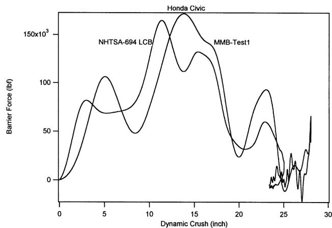
Figure 5. Comparison of Force-Deflection Curves for NCAP-694 Load Cell Barrier Test and MMB Test on the Honda Civic.
