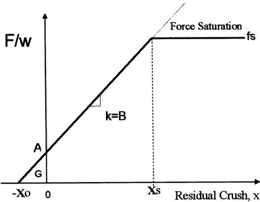
Figure 0. Force Saturation Model Notation.
