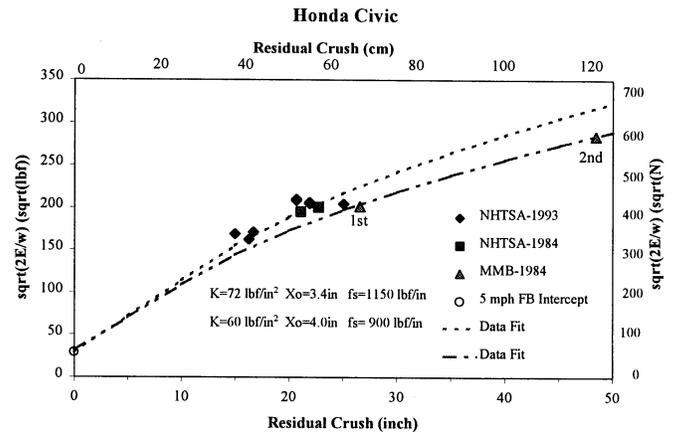
Figure 6. Crash Plot ( $\sqrt{2E/w_c}$  vs Residual Crush) of the Honda Civic Frontal Test Data.
