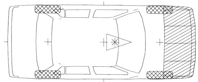
Figure 7. Honda Civic Damage Profile after 1<sup>st</sup> Impact
