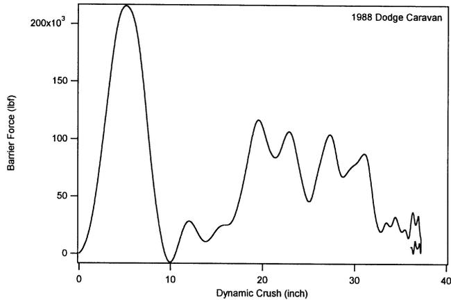
Figure 12. Observed Force-Deflection for Rear Impact of a 1988 Dodge Grand Caravan (Extreme values exaggerated by MMB accelerometer motion).
