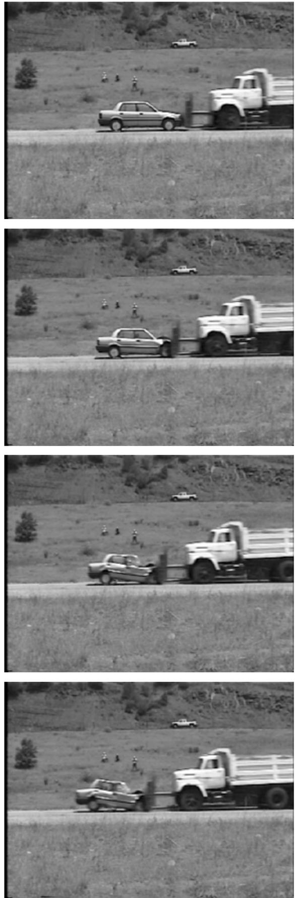
Figure 1. Frontal Crash Test of the MMB with a 1984 Honda Civic.
