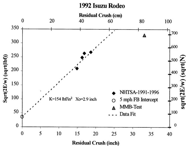
Figure 17. Crash Plot for Isuzu Rodeo Offset Override Impact.
