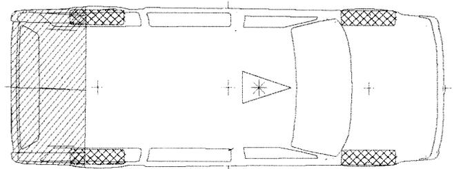
Figure 14. Damage Profile at the Rear of a 1988 Dodge Grand Caravan.
