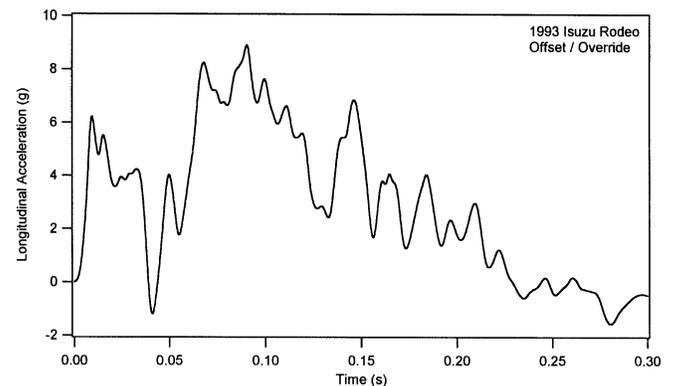
Figure 16. Isuzu Rodeo Average Longitudinal Acceleration.
