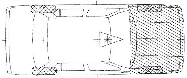
Figure 10. Honda Civic Damage Profile after 2<sup>nd</sup> Impact.
