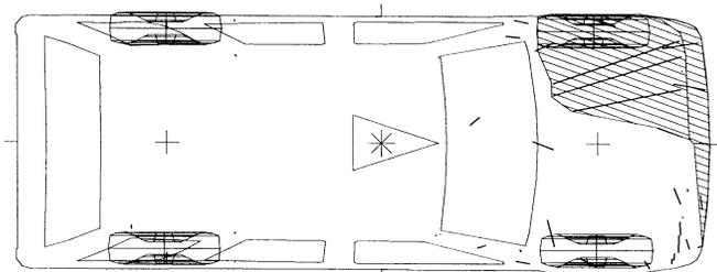
Figure 18. Damage Profile at the Left Front of a 1992 Isuzu Rodeo
