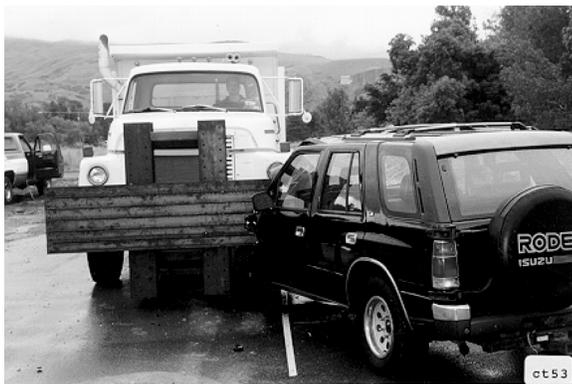
Table 4. Frontal Offset Override Impact Test; 1992 Isuzu Rodeo with MMB
