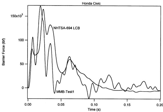
Figure 4. Comparison of NCAP-694 Load Cell Barrier Force time-history with MMB Force on the Honda Civic.
