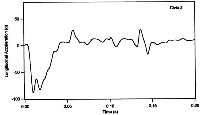
Figure 9. Acceleration of the Honda Civic During the Repeated Impact.
